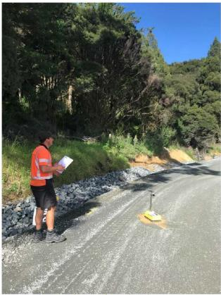
Figure 21: Section Four Nuclear Density Testing
