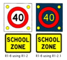
unlit. For signs that display only the 40km/h variable speed limit and are blank for the rest of the time, the roundel is displayed with red, lit pixels. Alternatively, for signs that display the permanent speed limit at times when the variable speed limit does not apply, the roundel may be displayed with either red, lit pixels or with red retro-reflective material.
