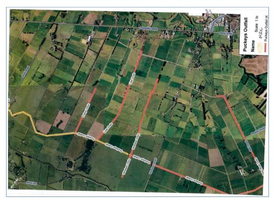
The following map is an example of Matthews Outfall County Drain which illustrates urban stormwater flowing into Land Drainage drains. It illustrates how urban stormwater flows into Drainage District Drains to get into rivers:
