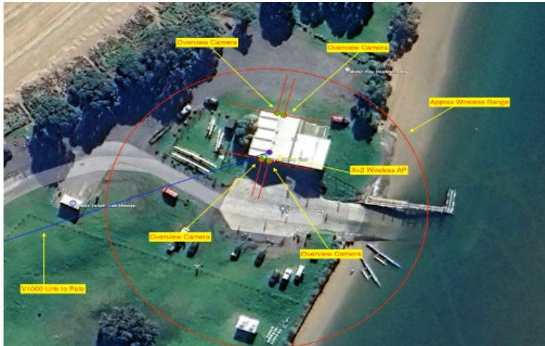
Figure 9: CCTV: 4 cameras and Public Wi-fi to be installed at the Yacht Club, requirement for power and fibre (tor connectivity) and ability to house equipment from the Yacht Club, has been provisionally agreed.
