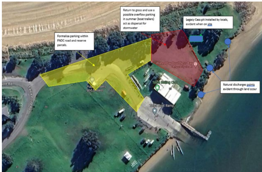
Figure 6: Stage 2_Drainage & stormwater work and designated car & boat parking.
