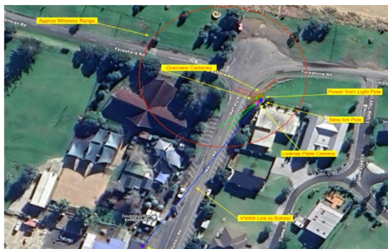
Figure 11: CCTV: 2 cameras and Public Wi-fi to be installed on pole on Foreshore Road/cnr of Mamaru Road, requirement for power and fibre (for connectivity) and ability to house equipment, which will be securely located nearby.
