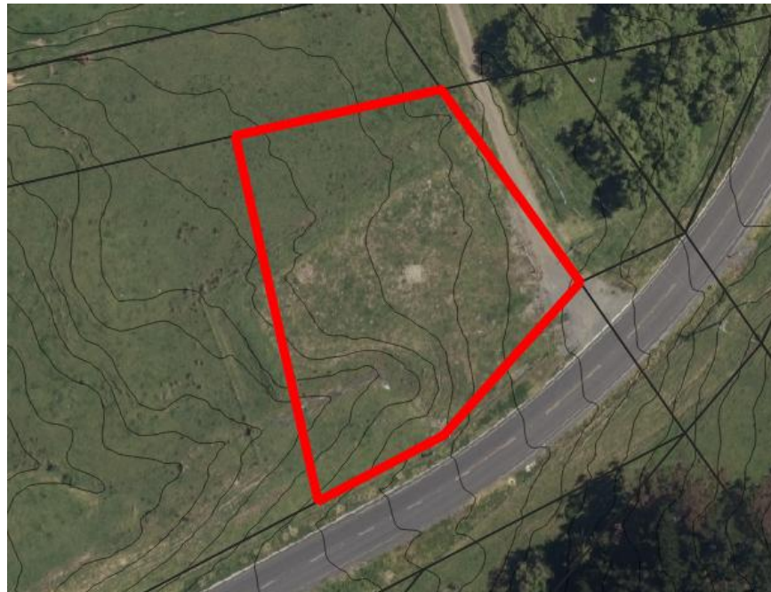
Figure 21 De Thierry Street, 2018 LiDAR data and aerial image from 2015 Property boundary indicative only outlined in red, contours are shown at 1m intervals, Image courtesy of NRC, 2015.
