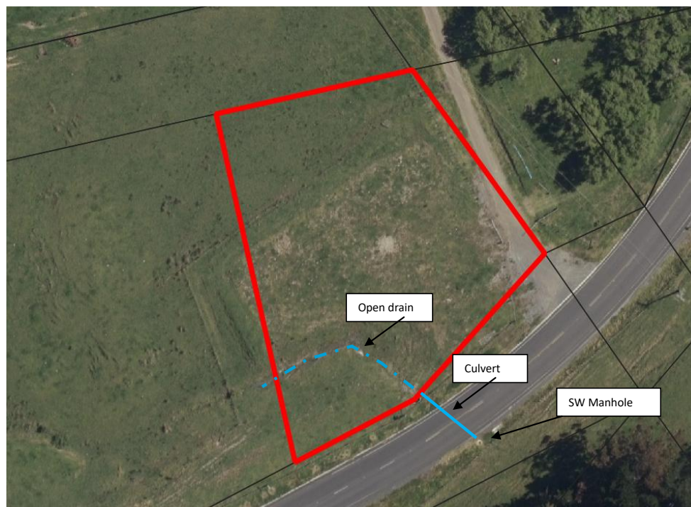
Figure 23. 19 De Thierry Street, Rawene, Inferred stormwater reticulation Property boundary indicative only (red), inferred location of stormwater manhole, culvert and open drain, image courtesy of LINZ
