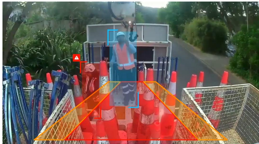
Figure 1 Camera with AI technology has identified worker movement (in red) on the left and alerted the driver that a person has not attached their harness yet.
