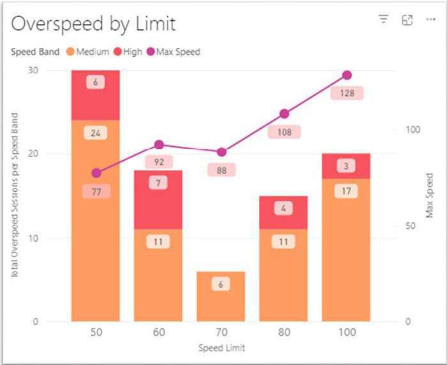
Figure 3: The data used in the graph above is taken from eRoads and shows overspeed events in comparison to road speed limits for Q1 2022. During Q1 the fastest speed recorded was 128kph in a 100kph zone. The highest % speed over a limit was 54% as a result of a vehicle recorded driving at 77kph in a 50kph area.
