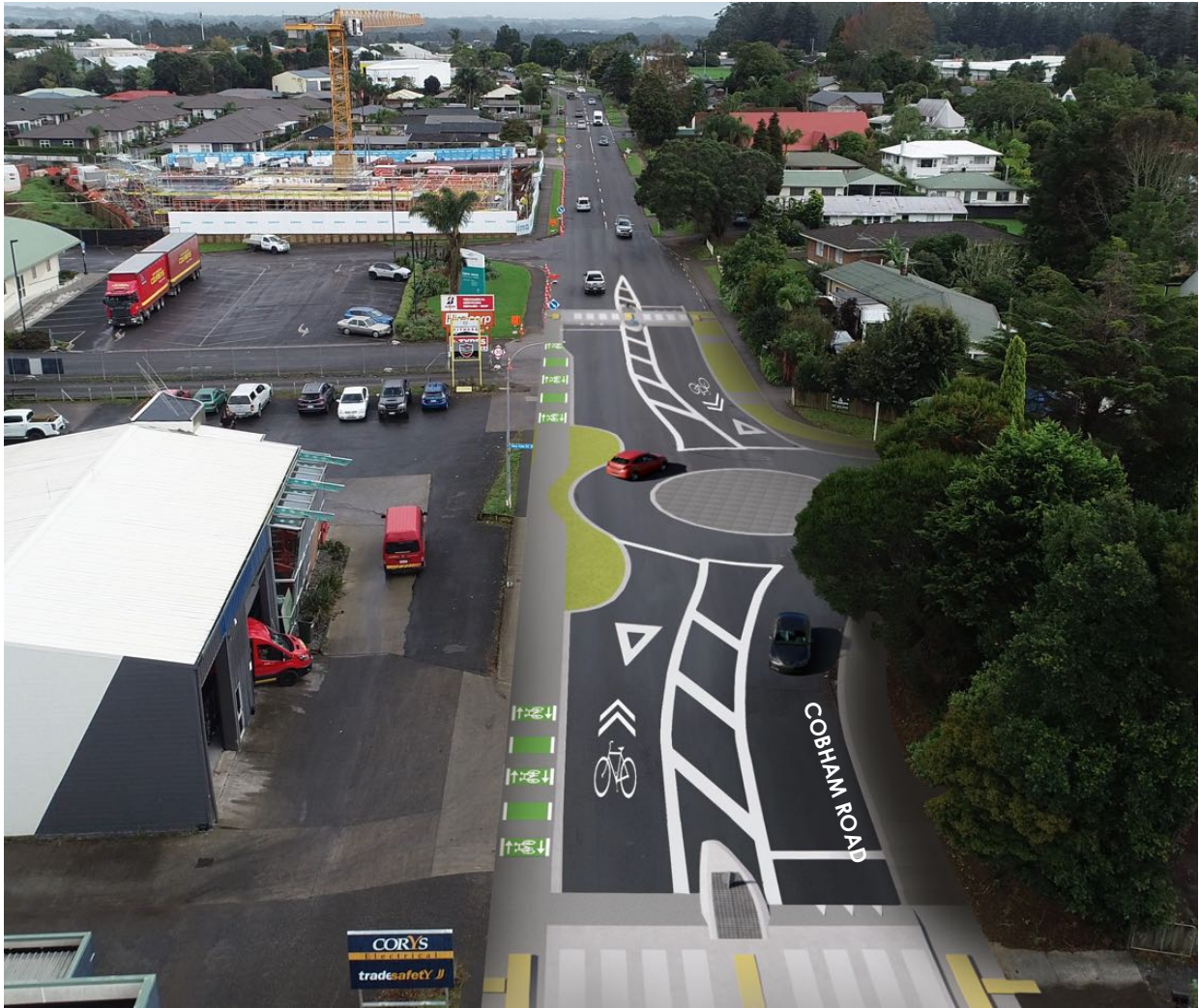
C. INTERSECTION IMPROVEMENTS PROPOSED WITH ROUNDABOUT AND RAISED ZEBRA CROSSINGS
