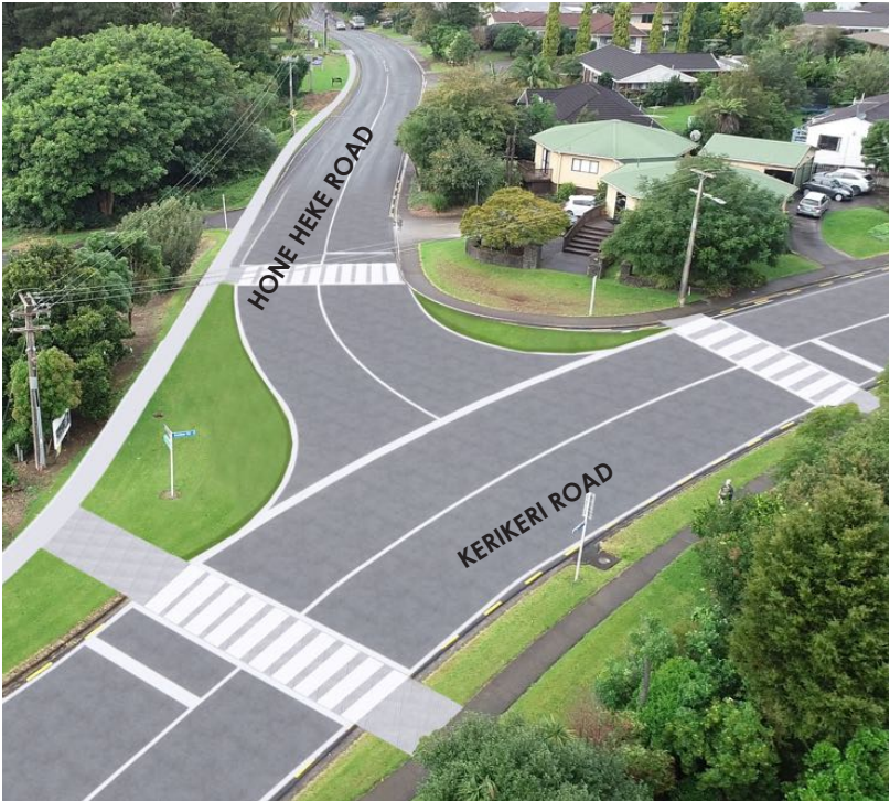
C. INTERSECTION OPTION 1 INTERSECTION IMPROVEMENTS PROPOSED WITH NARROWER TRAFFIC CORRIDOR, PEDESTRIAN CROSSINGS AND NEW SHARED PATH
