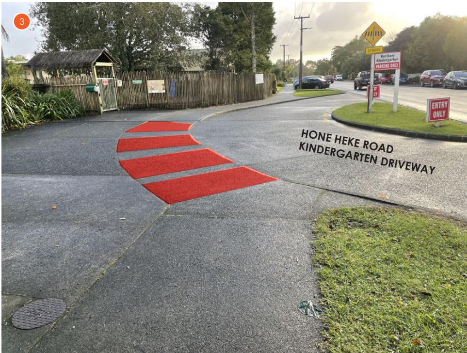
C. PROPOSED RED SURFACING IMPROVING PATH VISIBILITY FOR DRIVERS
