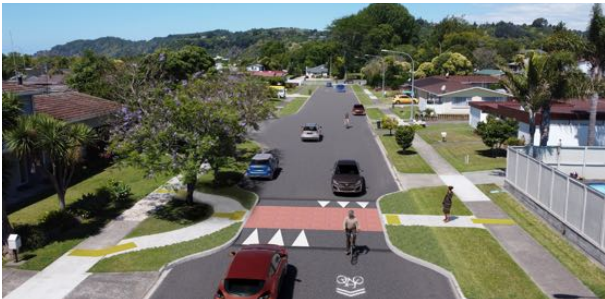
D. KERB EXTENSIONS, RAISED COURTESY CORSSING/ SPEED PLATFORM - SPECIFIC TREATMENT OPION TO BE DETERMINED IN CONSULTATION WITH RESIDENTS
