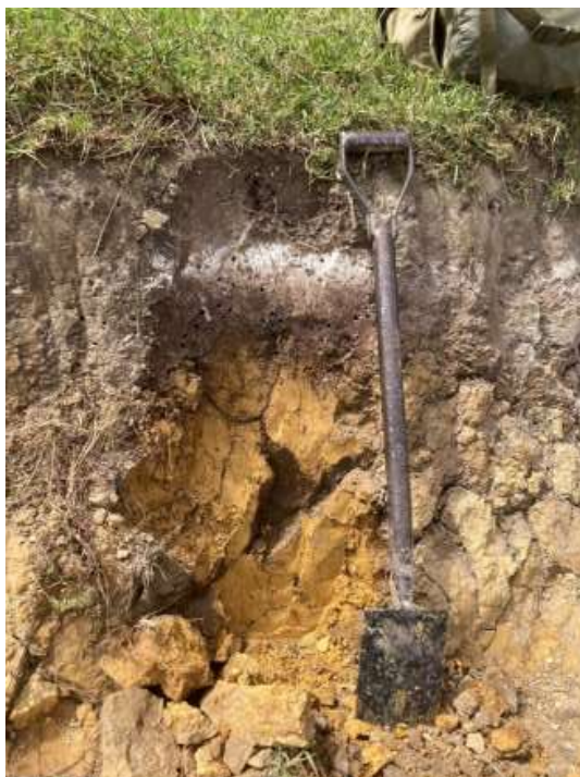
Figure 11. Photo of sampling location 1099 at Site 13 showing presence of pale E horizon and clayey subsoils.
