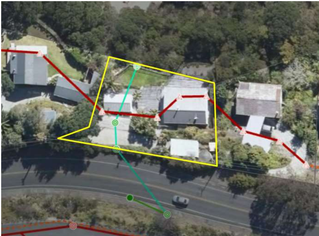
Figure 1- Existing Reticulation. Red Wastewater, Green Stormwater
