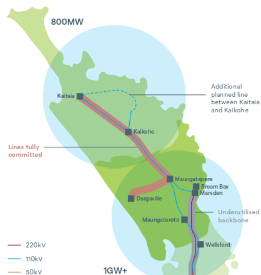
Figure 7: Generation interest in Northland region and lines reaching capacity limit
