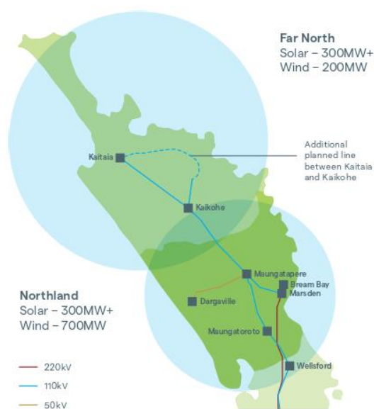
Figure 6: Estimated grid scale wind and solar resource availability
