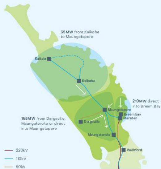
Figure 8: Illustration of existing network export capacity
